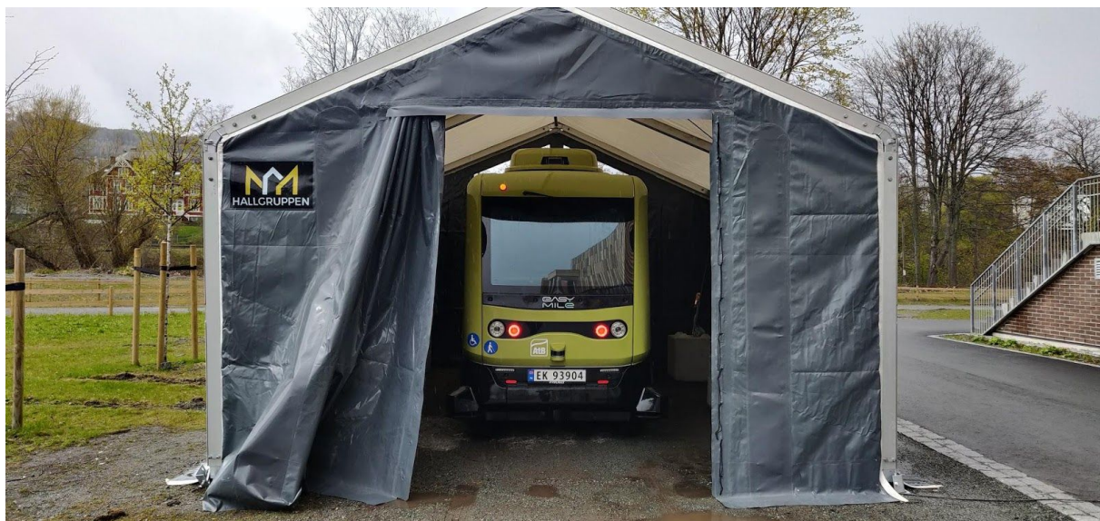
The self-driving bus in its garage tent, where it is charged and stored
