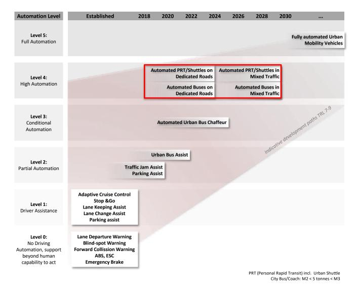
Figure 9: The Automated Driving development path for urban mobility vehicles
