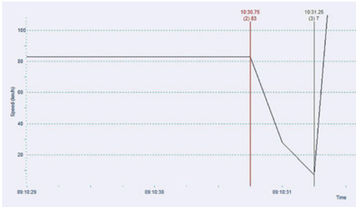
Figure 18: Speed recording from the truck's tachograph. (Source: police accident report)
