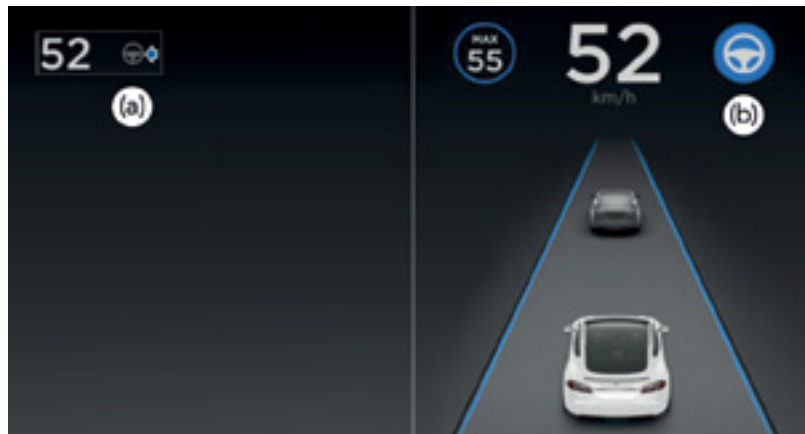
Figure 27: (a) If Autopilot is available, a grey Autosteer icon is displayed on the instrument panel. (b) The icon turns blue when Autosteer is engaged. (Source: Tesla Model S user manual 167 )
