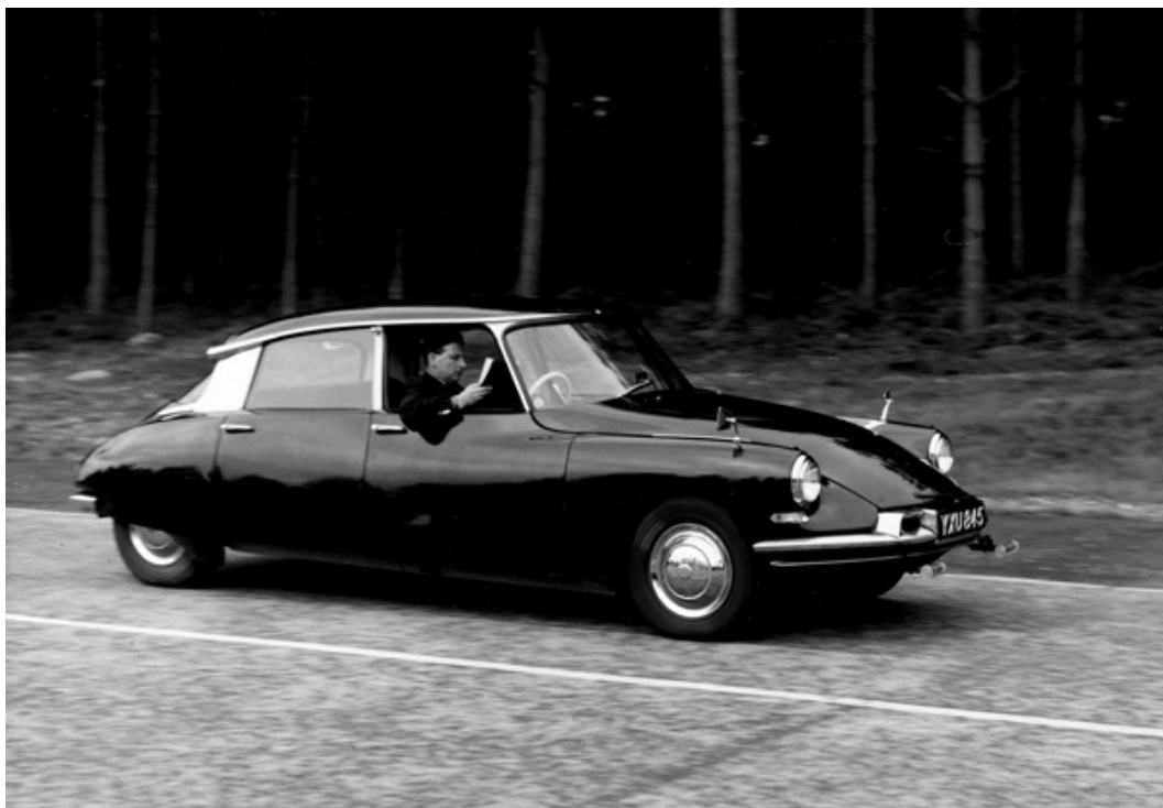
Figure 1. Citroen DS fitted with sensors and systems that enabled automated driving by following an electric guidance cable buried in the test track at the UK's Road Research Laboratory (picture credit: TRL Limited).
